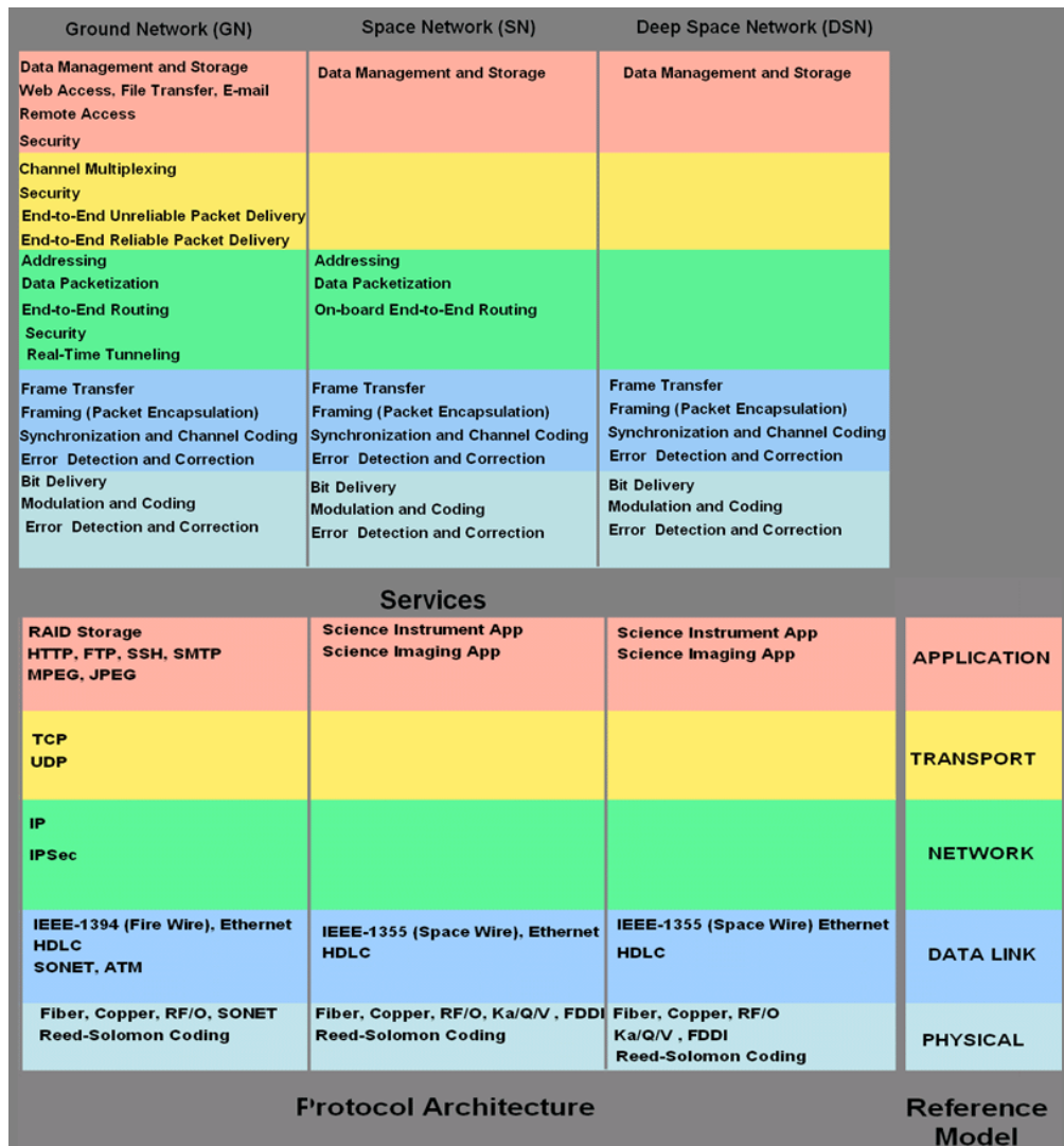
Fig.11: The Abstract NASA Backbone Network Protocol Architecture.
