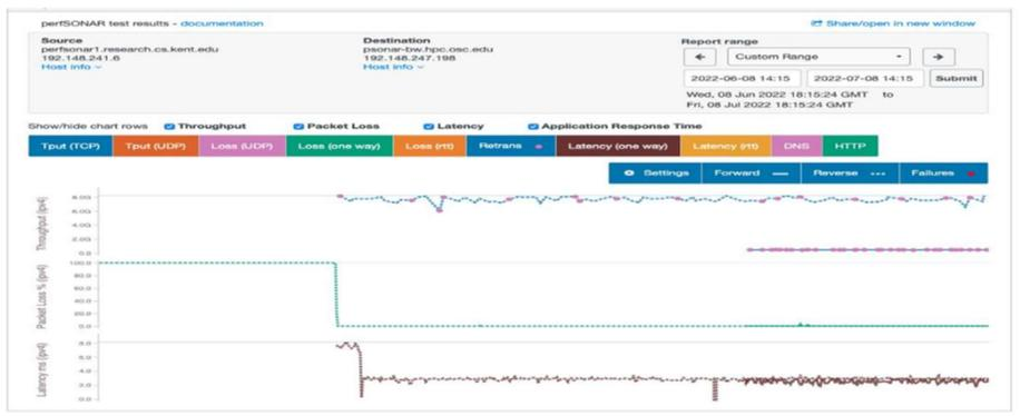
Fig. 10. PerfSONAR Results DTN Network to Ohio Super Computer
